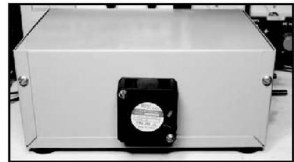
Figure 4 — View of fan mounting arrangement on one side of the aluminum box.
