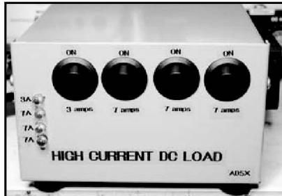
Figure 6 — Front panel view showing control and indicator layout.
