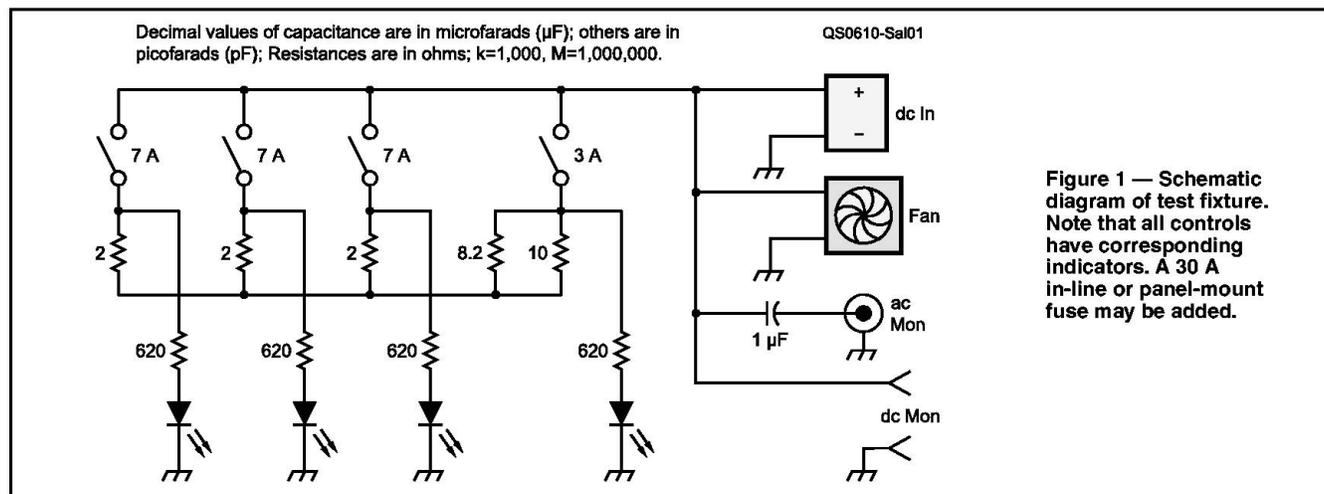
Figure 1 — Schematic diagram of test fixture. Note that all controls have corresponding indicators. A 30 A in-line or panel-mount fuse may be added.
