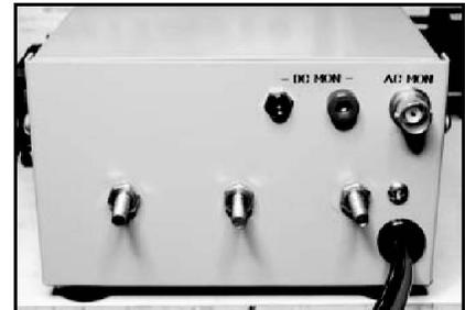
Figure 7 — Rear panel with connectors.
