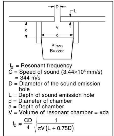
Figure 19—Here's the fundamental approach to constructing a resonator to improve the loudness and purity of the buzzer's tone. The resonant frequency ( $f_0$ ) should equal twice the frequency of the buzzer to increase sound pressure. Do not make dimension D too small, or the acoustic resistance will increase. The equation is a starting point; experimentation will optimize your results (see text). Dimensions are in millimeters unless otherwise noted.
