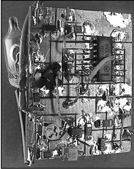
Figure 16—A top view of the SM version of the timer described in the text. The 3-V battery that powers the circuit is mounted on the bottom side of the board.
