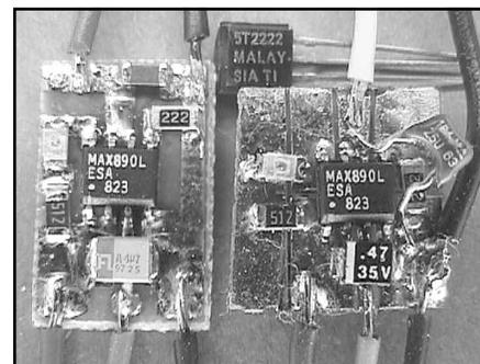
Figure 7—Here are two versions of the SmartSwitch compared in size to a TO-92 package transistor. The board on the right is homemade; the one to the left is available from N4UAW; see Note 11.
