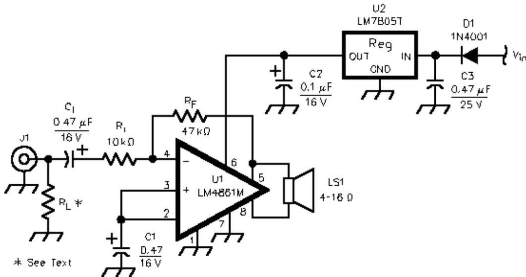
Figure 1—Schematic of the SMALL amplifier.
