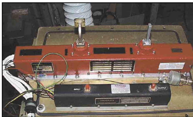
Figure 7—An 80-W 32-38-GHz Varian TWT; a Hughes 10-W TWT and glass 2C39 tube.
