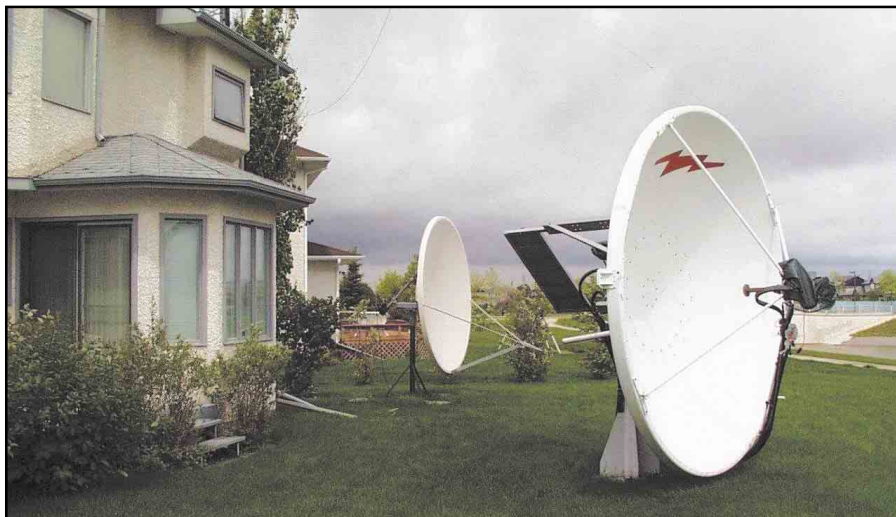
Figure 1—The 3-meter Andrew prime focus and 2.4-meter offset feed dishes at VE4MA.
