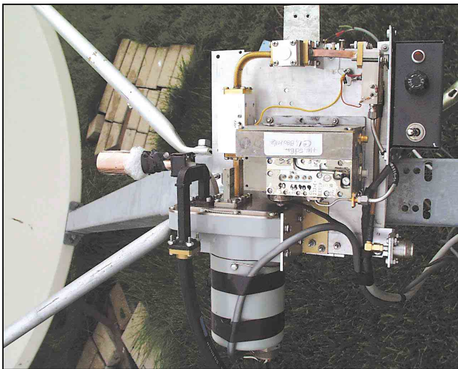
Figure 2—A 24-GHz feed assembly (receive converter and waveguide switch) and W2IMU feedhorn.
