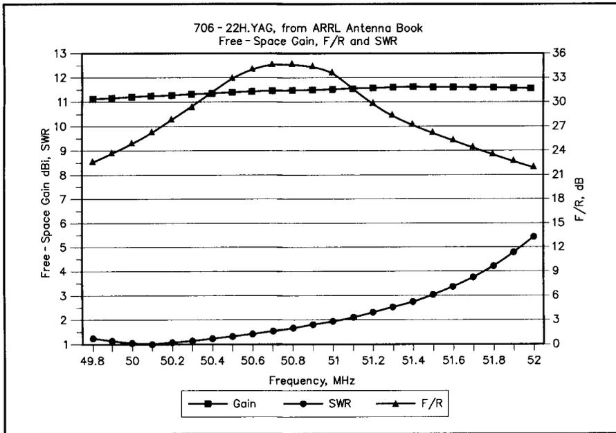
Figure 1—Graph of gain, F/R (front-to-rear ratio) and SWR over the 49.8 to 52.0-MHz range for 706-22H Yagi from *The ARRL Antenna Book*. The gain peaks at 51.6 MHz; the F/R peaks at 50.7 MHz. The matching network has been adjusted for a 1:1 SWR at 50.1 MHz.
