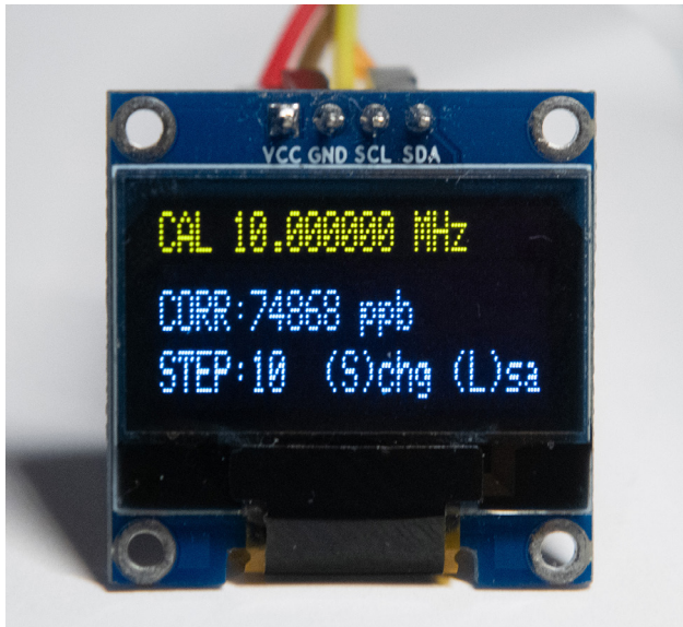
Figure 2 — Calibration mode display during 10 MHz reference adjustment.
