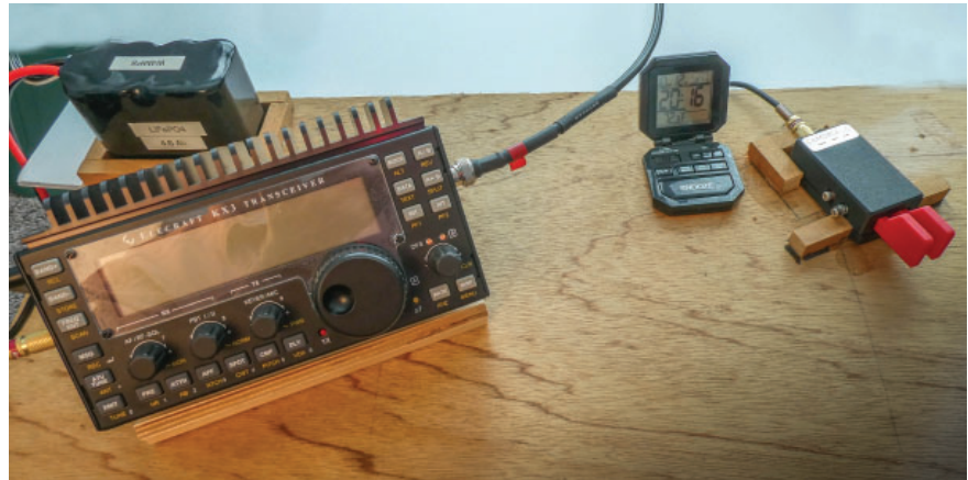
Marc's "Shack on a Board," consisting of an Elecraft KX3 transceiver, portable key, UTC clock, and 4.6 Ah LiFePO4 battery, mounted to a lightweight piece of plywood.
