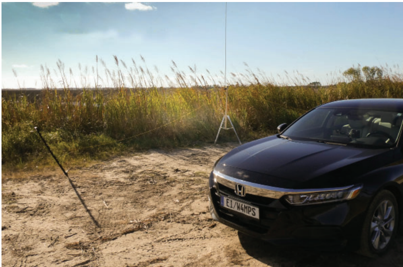
Marc, W4MPS, operates from Gull Rock Game Land (POTA US-6908) using his elevated 20-meter quarter-wave vertical antenna.
