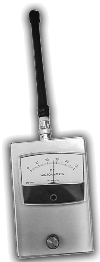
Figure 4.36 — A field strength meter is used to check relative performance of an antenna by measuring the electric field intensity.
