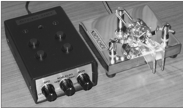
Figure 2.4 — An electronic keyer generates precisely formed and spaced dits and dahs under the control of a paddle. This combination makes it easy to send code at speeds over 15 words per minute (WPM) with much less effort.
