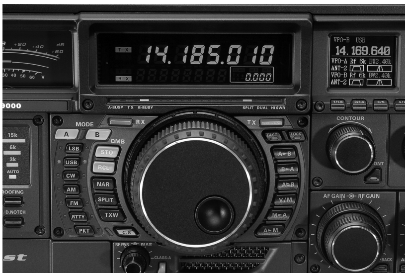
Figure 2.1 — The VFO control is usually front-and-center on a transceiver. It allows continuous frequency adjustments in small steps for smoothly tuning in signals.
