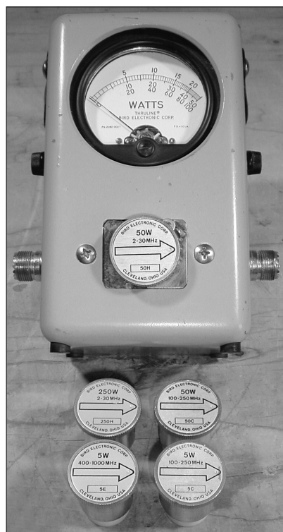
Figure 4.37 — The Bird Model 43 directional wattmeter uses sensing elements designed for a specific frequency range and power level. Forward and reflected power are read by rotating the sensing element. (One sensing element is plugged into the meter, and four other elements for different power levels and frequency ranges are shown below the meter.)
