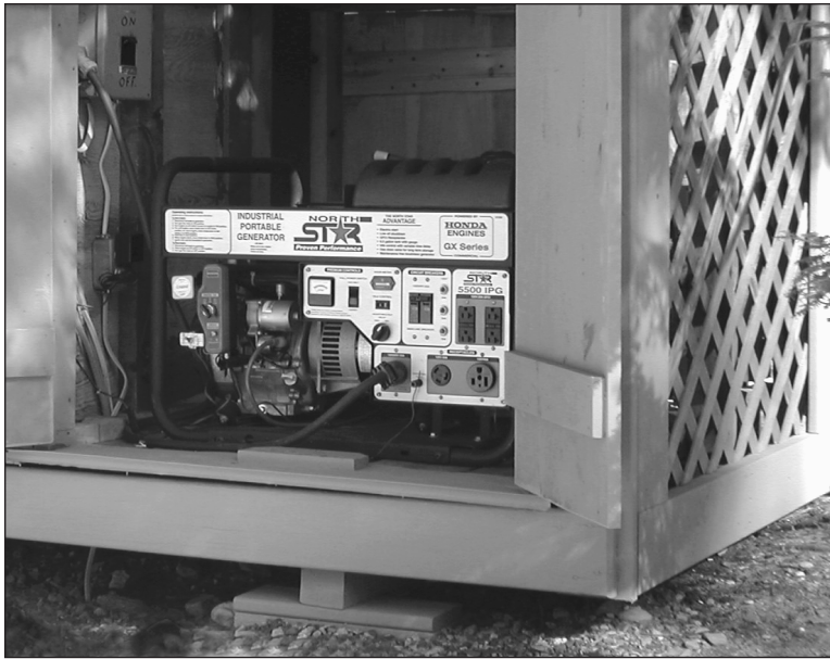
Figure 9.6 — Install your generator in a well ventilated area, away from living areas.
