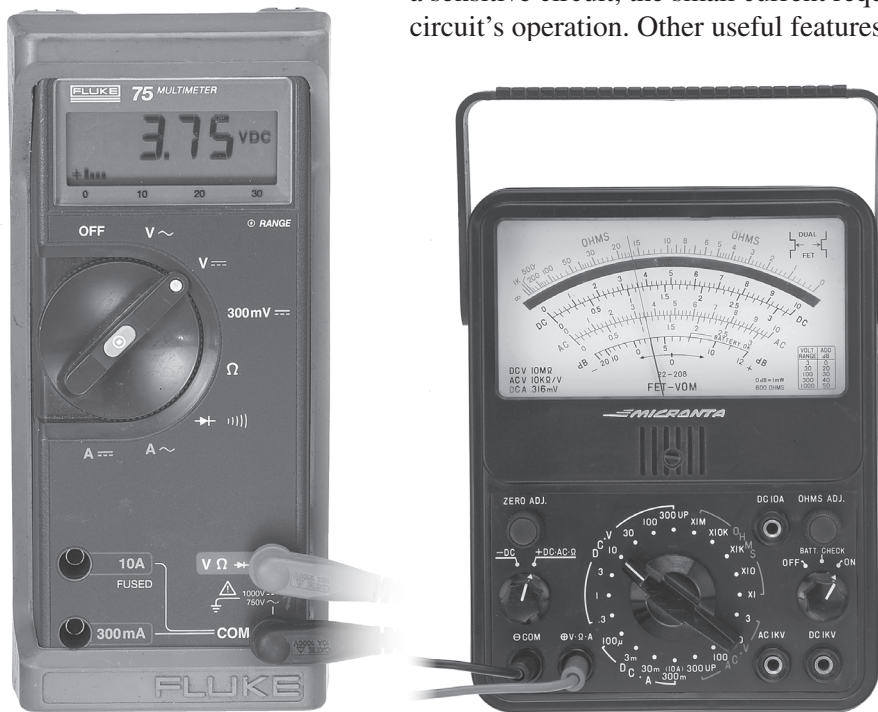
Figure 4.32 — A digital voltmeter (DVM) shown at the left provides precise measurements of voltage, current and resistance. Many models can also act as a frequency counter or component tester. Analog meters (right) are often preferable for tuning and adjustments since the needle's movement makes adjusting for a maximum or minimum quite easy.
