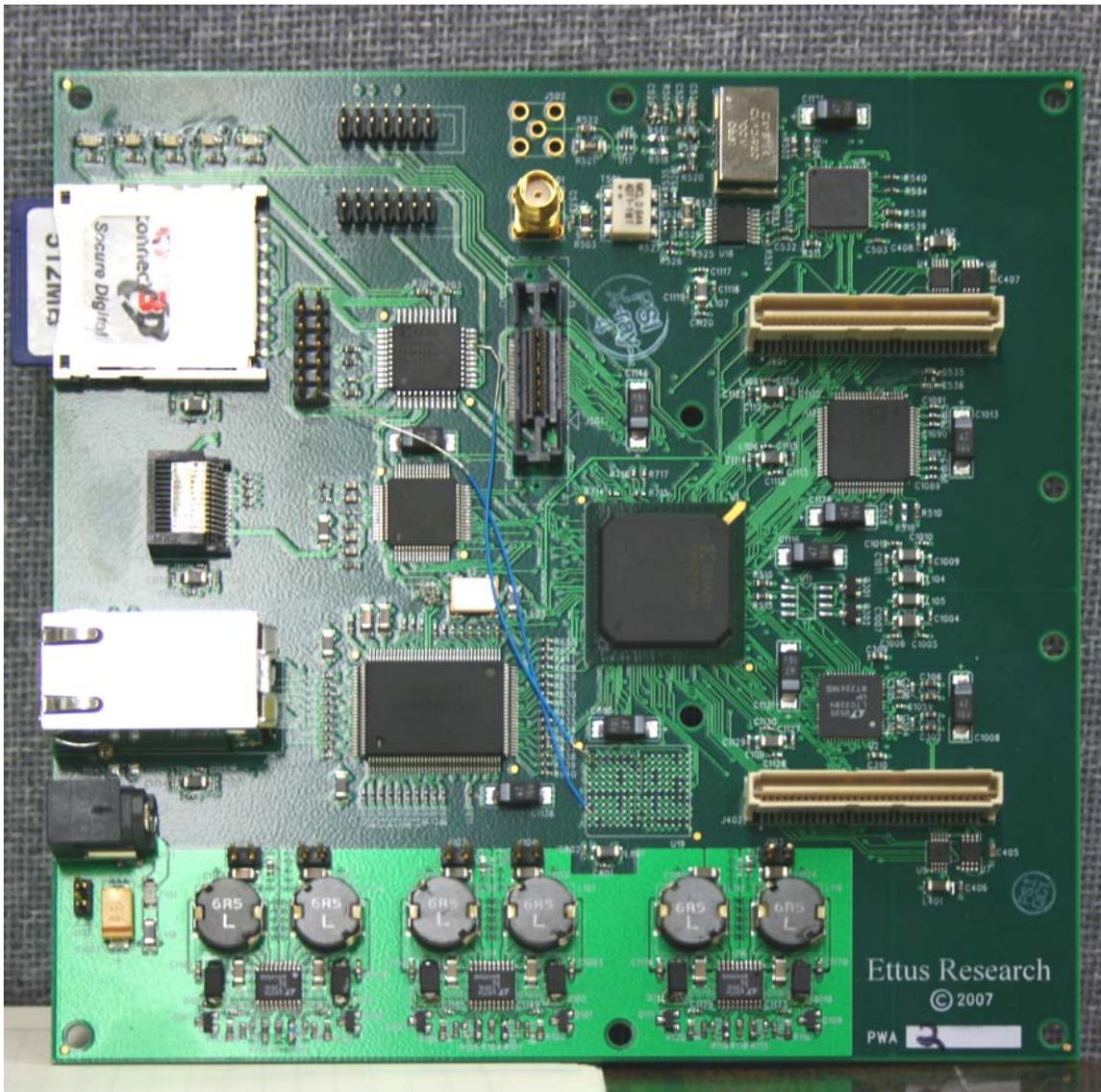
**Figure 6: Universal Software Radio Peripheral 2 (USRP2)**
