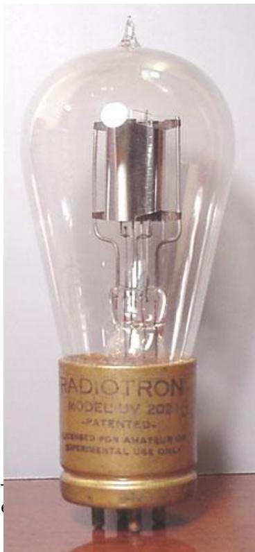
EARLY TRANSMITTER TUBE- RCA UV-202 5 WATT
