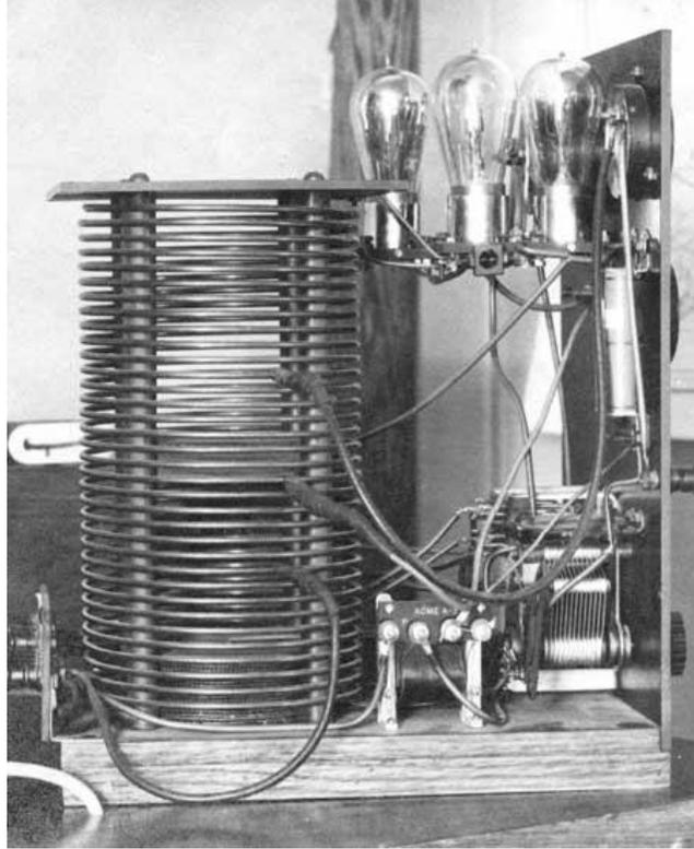
QUAD RCA UV-202 TUBES IN TRANSMITTER
